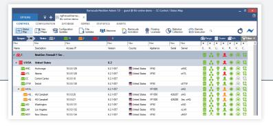
Status overview of a centrally managed Barracuda NextGen Firewall F-Series deployment
